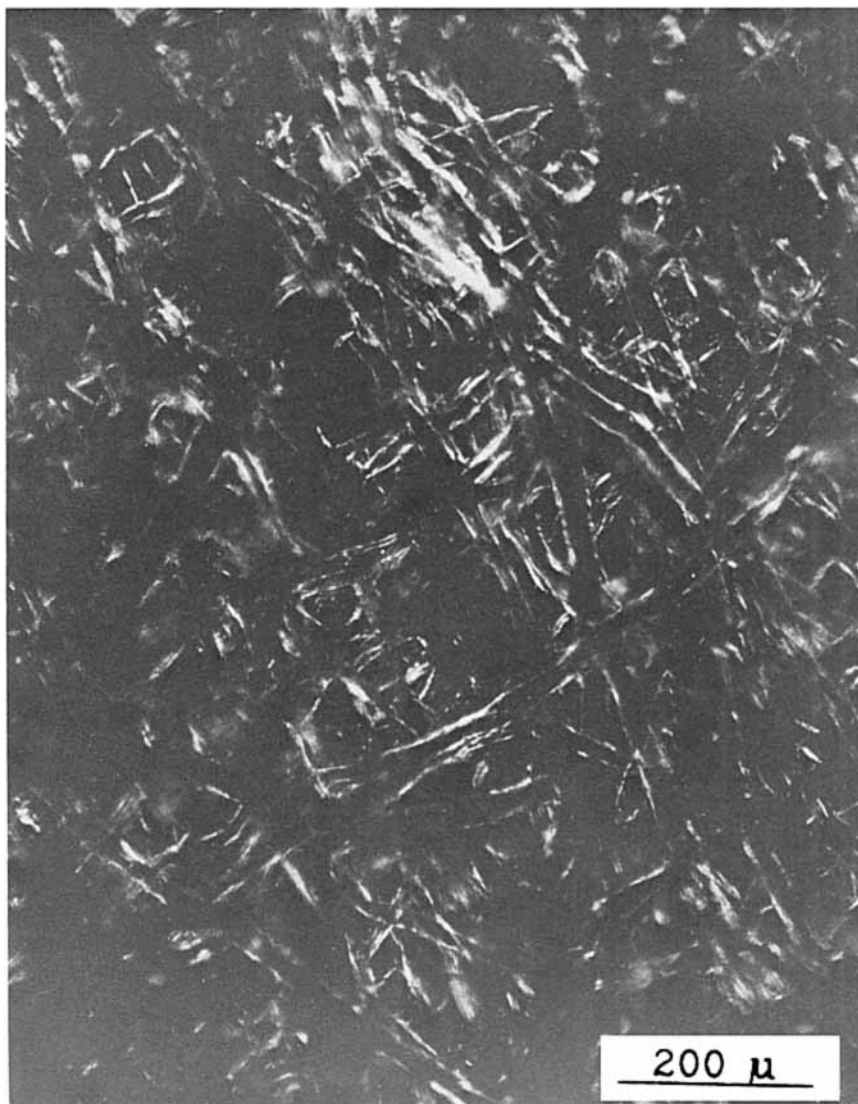
Fig. 5. Polyethylene residue after extraction of cellulose as seen in optical microscope under crossed polarizers.
